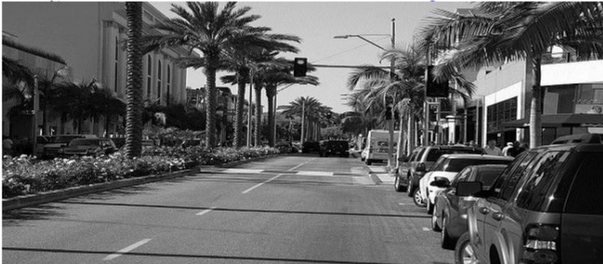
Figure 7. Maintain a minimum 18-inch offset between the face of median tree (at maturity) and the face of curb. Source: Dan Burden, walklive.org
