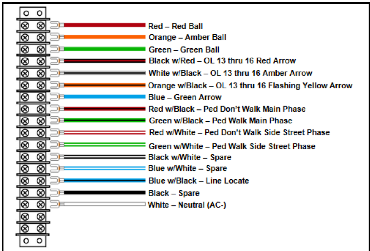
Figure 7.1: Terminal Block Layout for 16-Conductor Signal Cable
