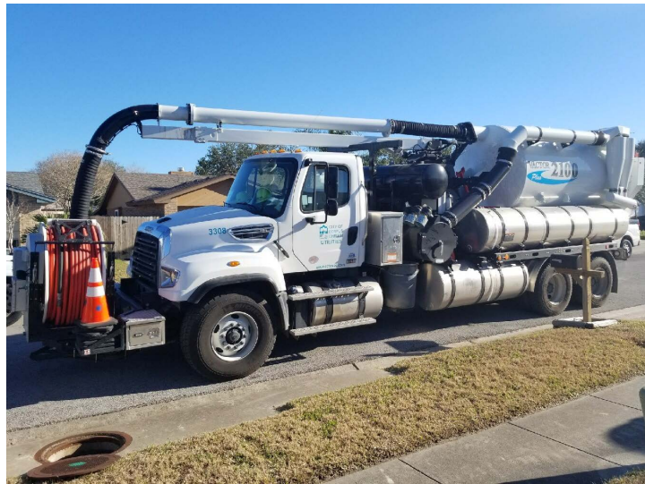
City vacuum truck is used to cleanup storm water inlets.
