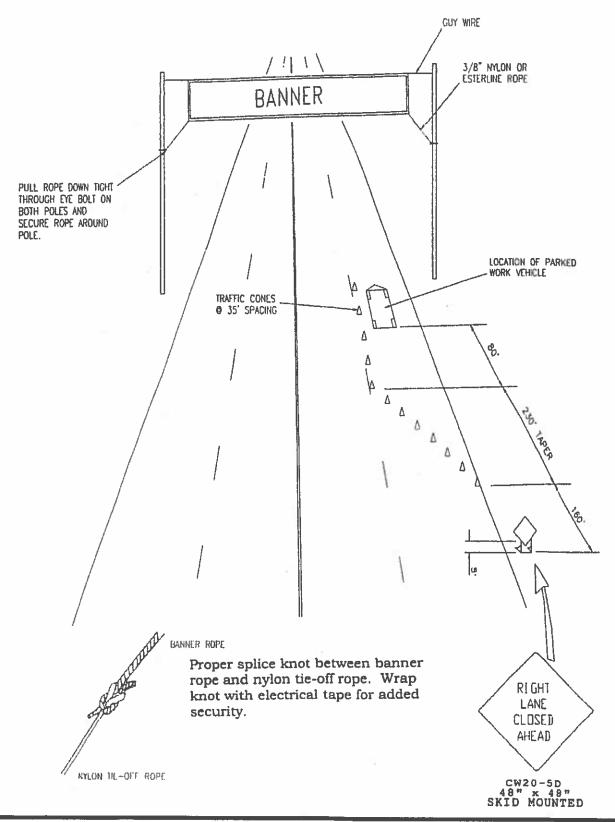
NOTE: Banner shall be approximately <u>4 feet high and 40 feet long</u>, supported by a steel guy wire at the top and a nylon or ester line role for banner tie-offs. Maintain minimum banner height clearance of 16 feet above street pavement.
