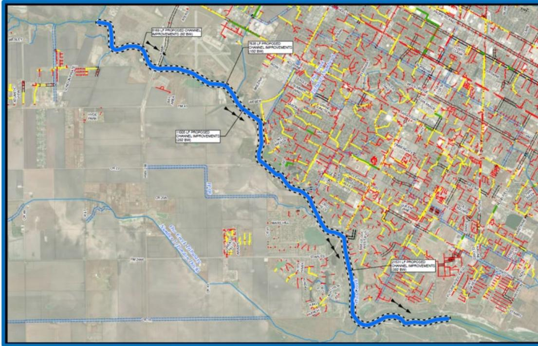
Channel improvements to widen and deepen main channel along centerline of Oso Creek from La Volla Creek confluence to Oso Bay to improve conveyance and provide additional capacity within the high banks of Oso Creek.
